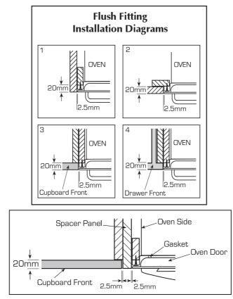
Cabinetry adjacent to ovens must have a minimum temperature rating of 90°C as stated in AS/NZS 3350.2.6 Page 2
